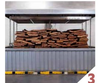
3 The planks are boiled in closed filtered stainless steel tanks. This process softens and cleans the material, while simultaneously expands and improves its internal structure.
