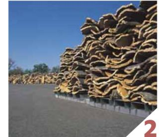
2 Cork is transported to an industrial plant, where it stays for at least 6 months, acquiring the ideal moisture content for processing.
