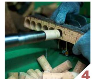
4 The planks to be used to produce natural cork stoppers are cut into strips and punched to extract the cylindrical stoppers.
