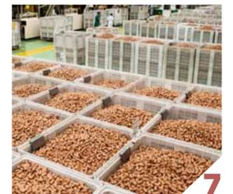
7 The final stages include: cleaning process with steam distillation, washing in an aqueous hydrogen peroxide solution, polishing and branding.
